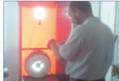
After the Icynene® application, blower door test data confirmed that this home met and exceeded the energy efficient requirements for designation as an EPA Energy Star™ Home.
